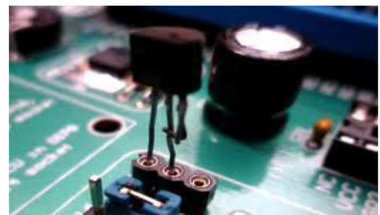
Fig 3 : Temperature sensor
