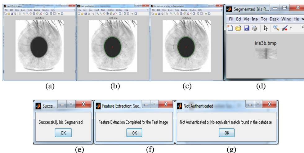
**Fig. 5:** Success in identifying the Unauthorized access (for not enrolled eye image “iris3b.bmp”). (a) Input Eye Image (b) Pupil Localization Stage (c) Iris regions selected for Segmentation (d) Segmented Iris Regions (e) Message showing “Successful Iris Segmentation” (f) Message showing “Successful Feature Extraction” (g) Message showing “Not Authenticated” or “No Match found” for unauthorized access to eye image “iris3b.bmp”.
