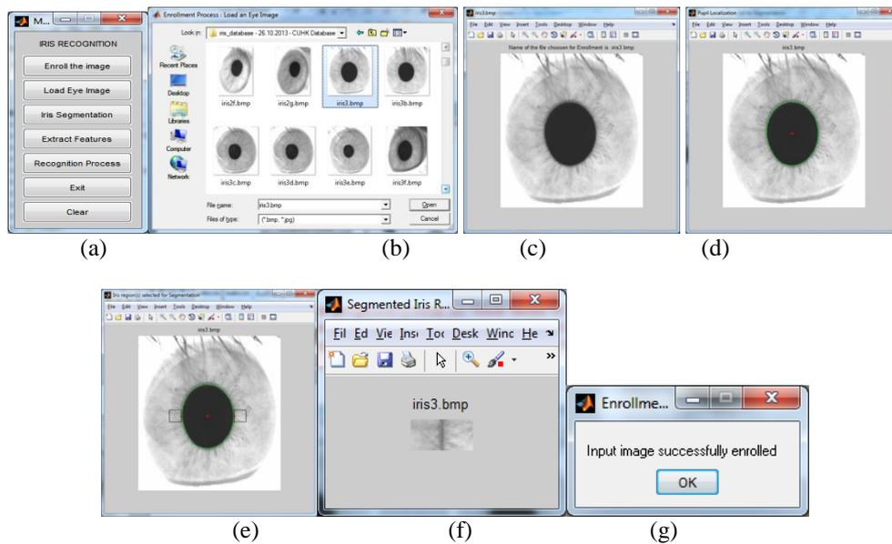
**Fig. 3:** Enrollment of sample eye image “iris3.bmp” in this proposed system (a) Main menu of the proposed system (b) Open dialogue box for choosing the Test image (c) Eye image “iris3.bmp” selected for Enrollment process (d) Pupil Localization Stage (e) Iris regions selected for segmentation by fixing the two special wedges over iris region (f) Segmented iris strip of 60 x 30 pixels size of eye image “iris3.bmp” (g) Message box showing the message “Input image successfully enrolled”
